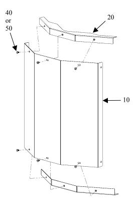
Figure 2. Assemble the Finishing Cover
